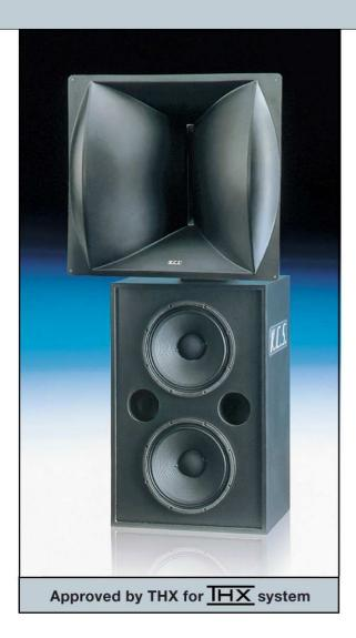
K.C.S. acoustic systems **S-3000** and **S-3001** are a high quality set specially designed as a screen channel group for large cinema theaters. These acoustic systems include a direct radiation technology bass cabinet with twin 15" Ø woofer. The treble system includes a compression driver with 4" Ø titanium membrane and 2" Ø mouth with a constant directivity horn.
