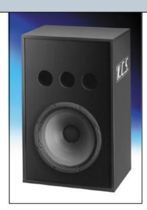
**C-118-H** consists of one K.C.S. S-1846 H 18" Ø woofer, with a high efficiency 4" Ø voice coil which has an excellent low-frequency response. This model features a high power handling capacity and reduced power compression. Using the direct radiation technology, this speaker provides a deep and highly linear bass sound.
